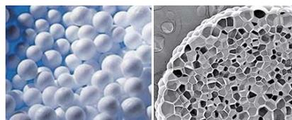
EPS foam particles (left), enlarged cross-section photo (right)
