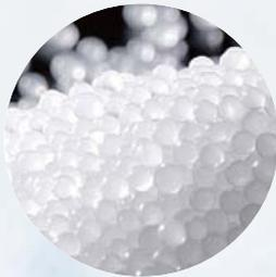
Raw material beads prior to foaming
